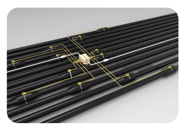
● 电缆温度传感器安装示意图 /Installation diagram of cable temperature sensors
