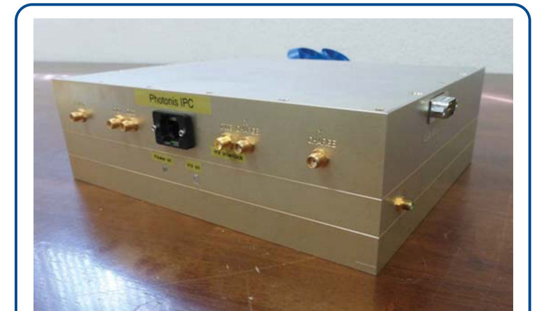
Figure 7: Parallel Cross Strip Electronics process the signals.
