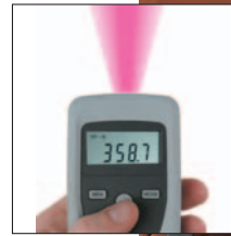
Non-contact (optical) rpm-measurement
