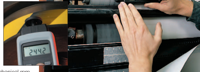
Mechanical rpm measurement on a roller
