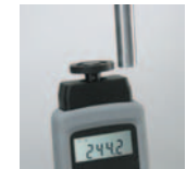
Mechanically with a surface speed disc
