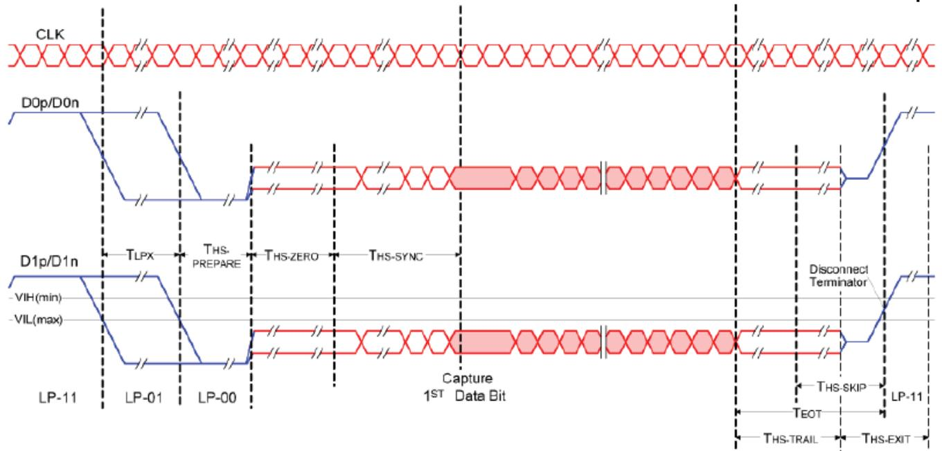
Note: THS-SYNC: Proper match found for Sync sequence in HS stream, the following bits are payload data.
