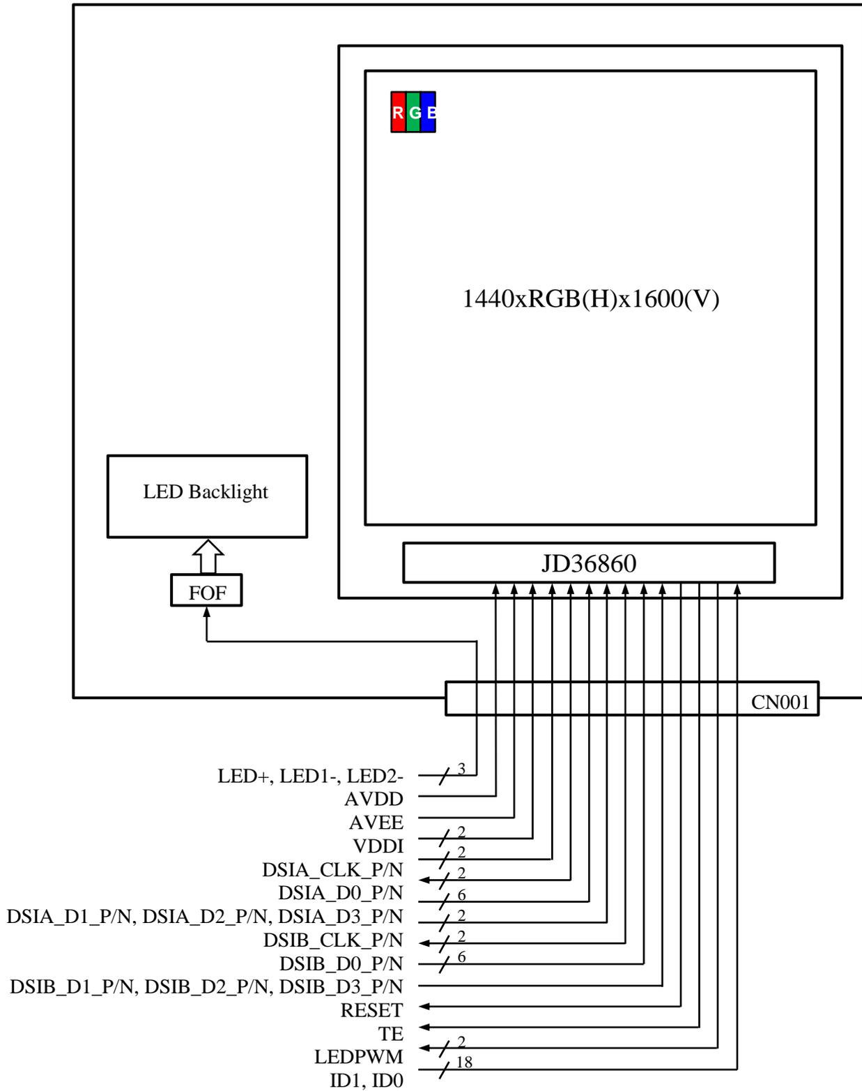
Note 1 LED Backlight Circuit Diagram
