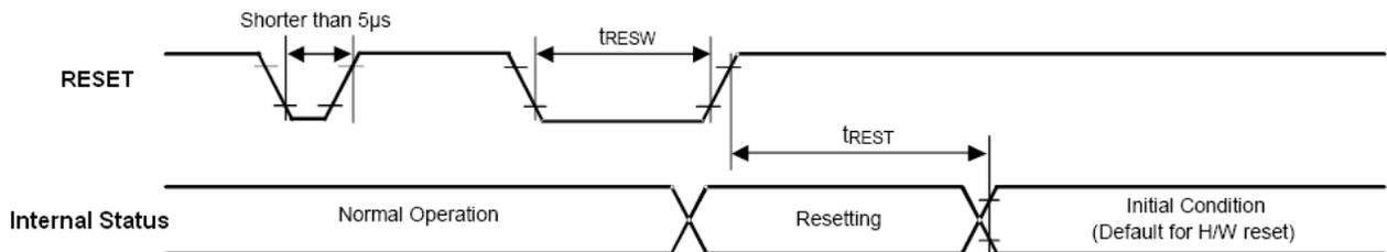
**Figure 5.4: Reset input timing**
