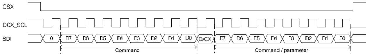
**Figure 5.4.1: Serial data write mode**
