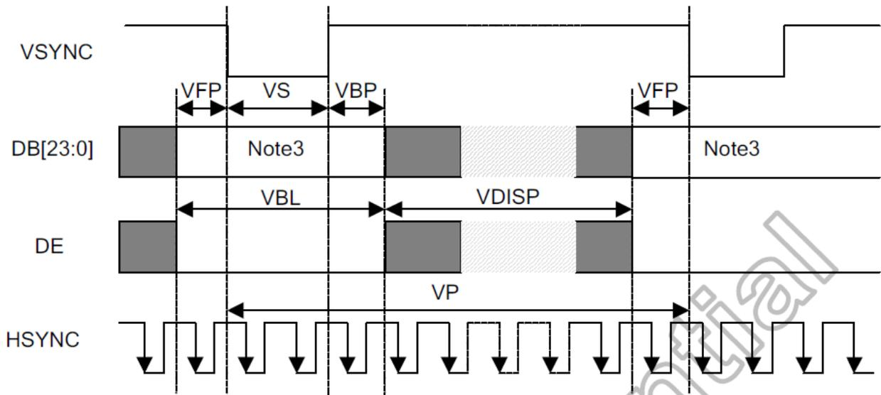
Figure 5.2: Vertical Timings for RGB I/F
