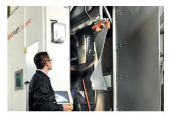
Very high end systems further increase controllability, with "selfmonitoring" wet blasting systems now available. Parameters such as pH, temperature, water and abrasive level, and air flow can be measured. With such extensive monitoring available the machines automatically dose themselves with more media, water or soap to ensure consistency, as well as recording trends and wear to help plan maintenance.
